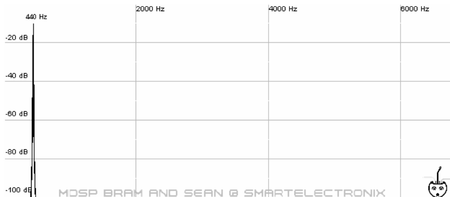
Figure 2. A 440 Hz sine wave and a graph representing its frequency and amplitude
